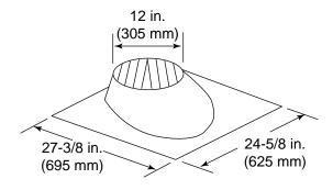
**RF370 Roof Flashing**
